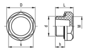
$\begin{array}{lll} D & = 32 \\ d & = G1/2 \\ h & = 11 \\ L & = 20 \\ M & = 20.5 \\ s & = 27 \\ Tightening (N m) = 8-10 \\ Weight (g) & = 8 \end{array}$
